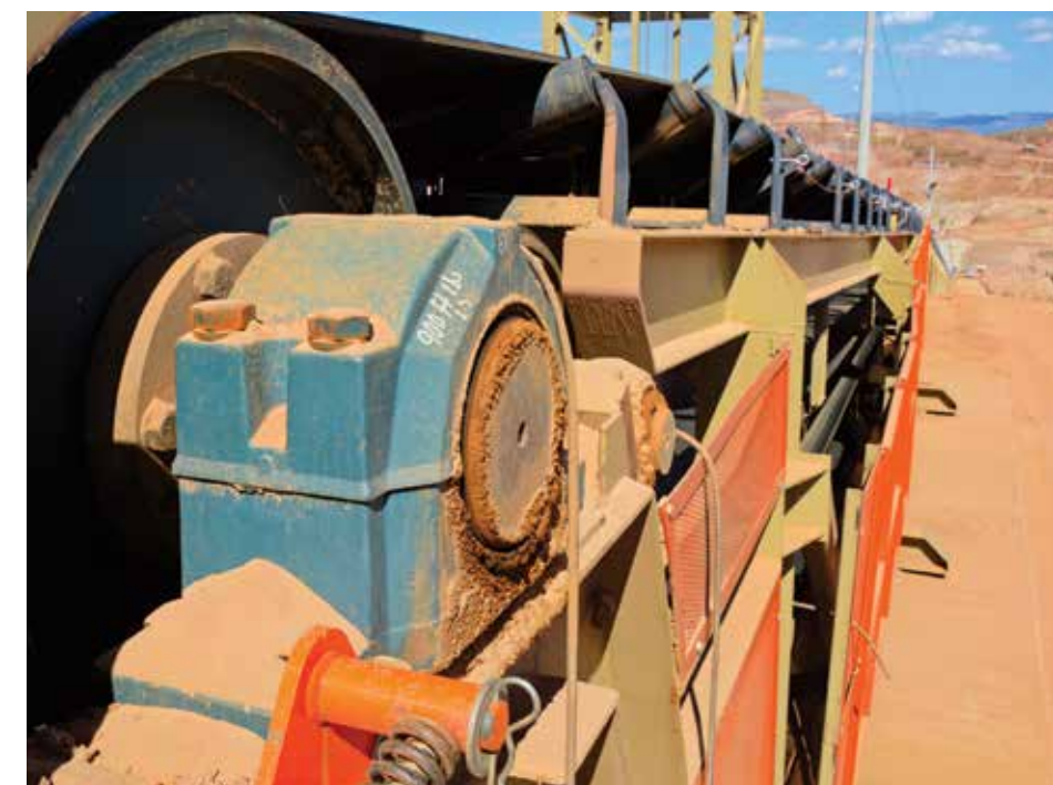
Baldor•Dodge USAF spherical roller bearings and Type E-Xtra tapered roller bearings were selected for the overland conveyors. Harsh-duty sealing systems will extend bearing life and increase reliability.
